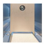
The pusher has a recess for the infeed conveyor belt. This means that very small products such as playing cards can also be processed.
