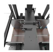
The product width is adjusted without tools using clamping levers and scales. With the help of the sensors on the sheet, the position of the band can be defined and the product banded once or twice.
