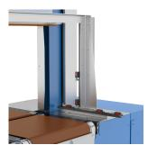
The sensors in the infeed enable the processing of different products, which are banded once or twice depending on their size. The sensors can be adjusted manually. **Technical specifications**
