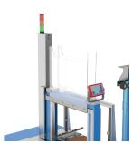
The pneumatic hold-down behind acrylic glass panes enables precise belt guidance and eliminates the need for additional casing.
