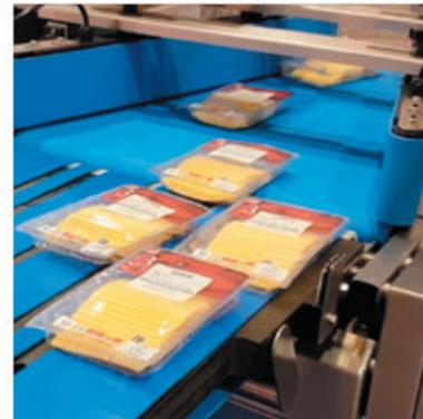
The Packleader BCS range of high speed convergers is designed to take multi-lane production of thermoformed packs and converge them at accurate spacing into a single lane.
