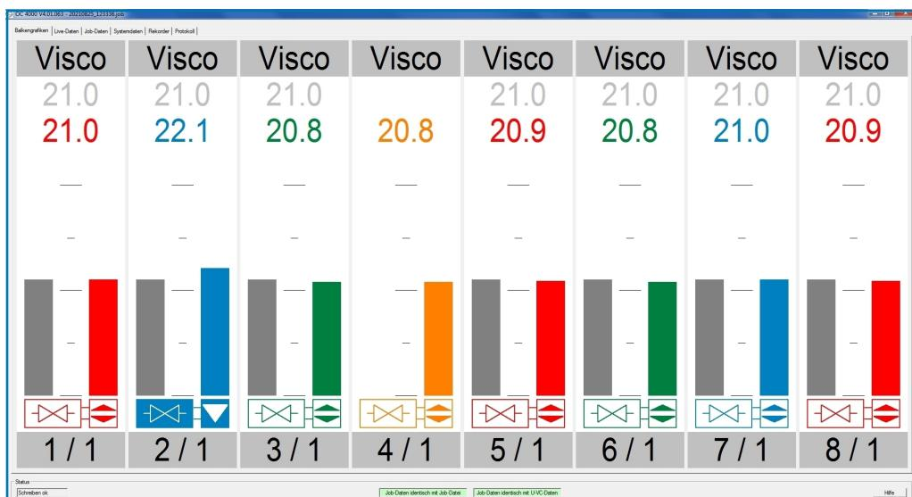
Software for easy visualisation, remote control and protocol functions for up to 12 connected UVC controls in an oc-Net - for viscosity and selected temperature channels/controls.
