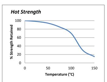
"Hot strength" shear strength tests performed on glass to mild steel. Fully cured specimens conditioned to pull temperature for 30 minutes before testing at temperature.
