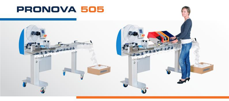
The Pronova 505 bagging machine is the smallest model in our range of standard machines. With a simpler design and fewer components than the other machines in the 500 series, it is particularly well suited for smaller growing productions that have packed manually into single bags and need to develop the packaging process to become a little more automated and much more efficient.
