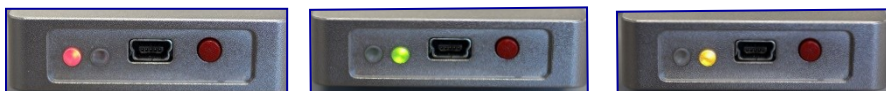
Different modes (Stop, Run, Pause) are indicated by the color of the LED
