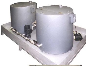
Heating tanks and coating-tray
